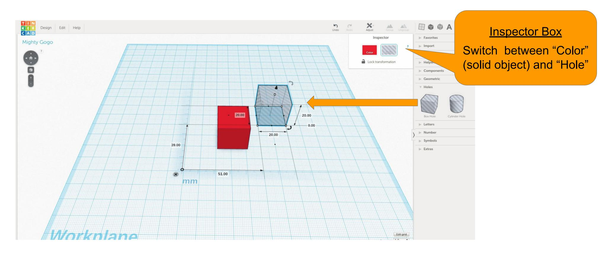
Let's say we want to cut a 10mm hole out of this 20mm box. First I will bring a **Box Hole** onto the workplane and resize it to 10x10x10 by typing in the measurement boxes (You may have to rotate the camera to see all the boxes).
